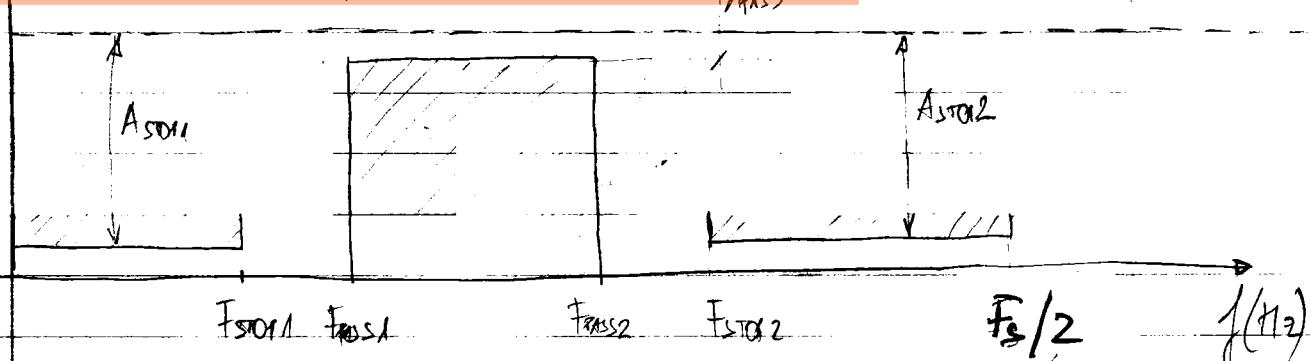
$A_{\text{STOP1}} = 60$ ; % ATTENUATION IN THE FIRST STOPBAND = 60dB
