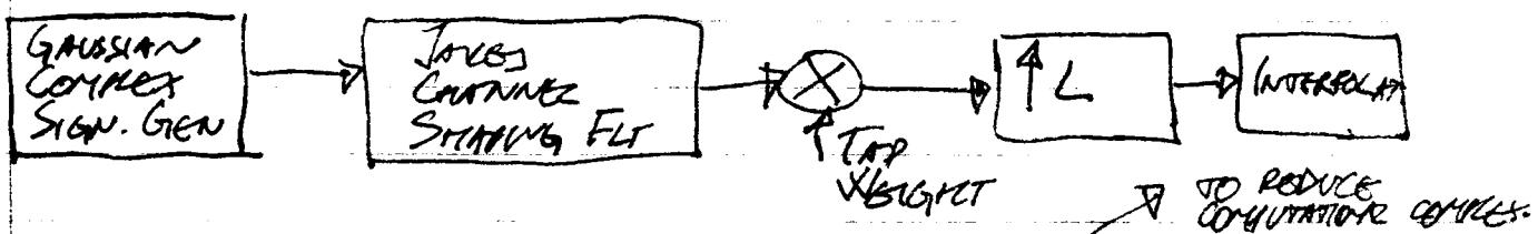
TAP-GAIN FUNCTION IS SAMPLED AT LOWER RATE, THUS INTERPOLATION IS REQUIRED
