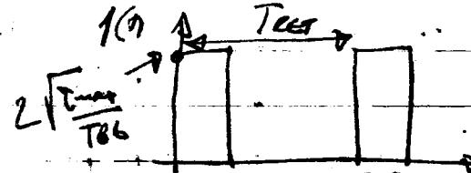
$$P(t) = 2 \sqrt{\frac{T_BW}{T_BB}} \quad 0 \leq t \leq T_BB \rightarrow \text{WIDEBAND PULSE}$$
