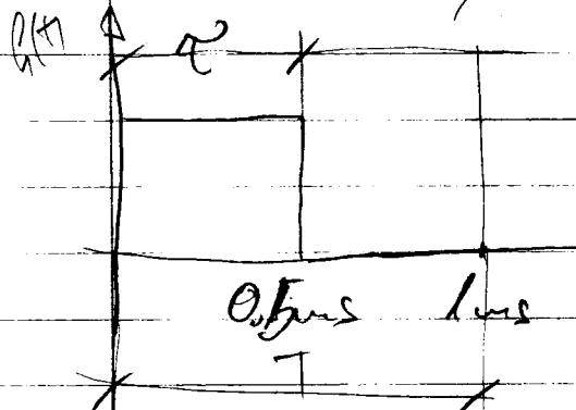
$$H(j\omega) = E \cdot T \frac{\sin(\frac{\omega T}{2})}{\frac{\omega T}{2}} = ET \frac{\sin(\pi f T)}{\pi f T}$$
