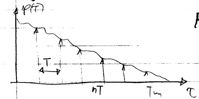
Figure: Sampled values of the power delay profile
