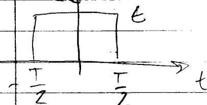
$$H(j\omega) = E \cdot T \frac{\sin(\frac{\omega T}{2})}{\frac{\omega T}{2}} = ET \frac{\sin(\pi f T)}{\pi f T}$$
